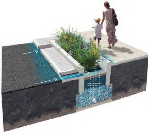
Diagram illustrating the opportunities for attenuation and surface water collection through rain gardens
